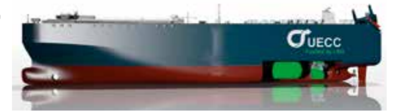
NEWBUILDING: Artist's impression of the dual-fueled Pure Car and Truck Carriers to be delivered to UECC in late 2016 in the Norwegian International Ship Register.
