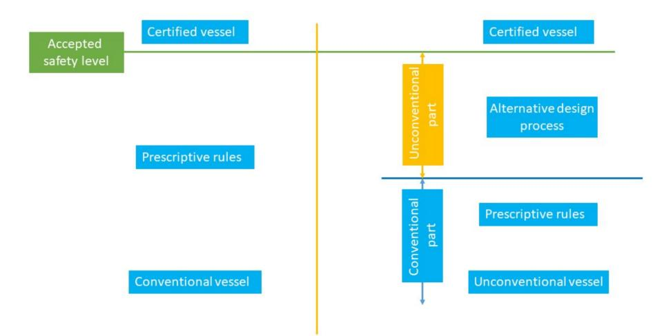
Figure 3: Flow chart for the certification process for conventional vessels versus unconventional vessels
