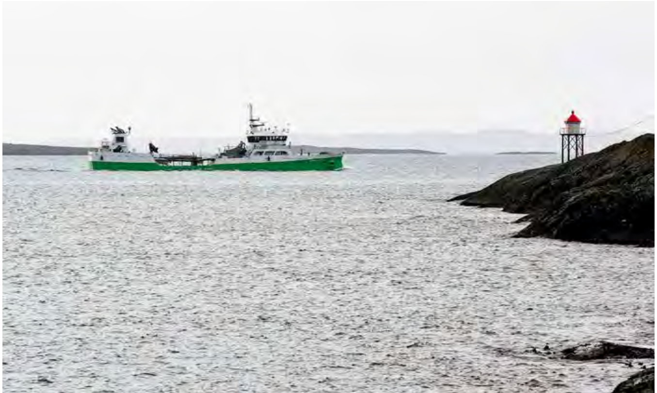
Øysund has a typical wellboat design with a low freeboard in loaded condition, which often leads to water on the main deck in rough sea. PHOTO:BJARTE AMBLE/NMA
