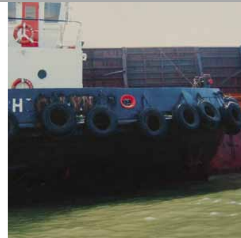
CHANGING THE IDENTITY of a ship is done by cutting the embossed name and repainting. ILLUSTRATION PHOTO: PRC
