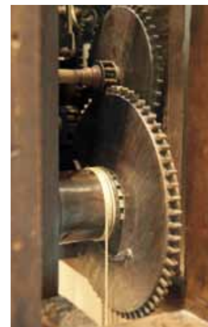
WOODEN CLOCK. John Harrison was a carpenter and made his first clocks out of wood, including the cogwheels and axels.
