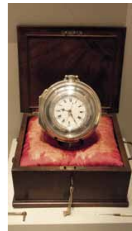
HARRISON'S LAST CHRONOMETER. H5 is Harrison's ultimate marine timepiece, seen here in its original case. Though simpler in external design than H4, H5 had better thermal compensation and was a more accurate timepiece.
